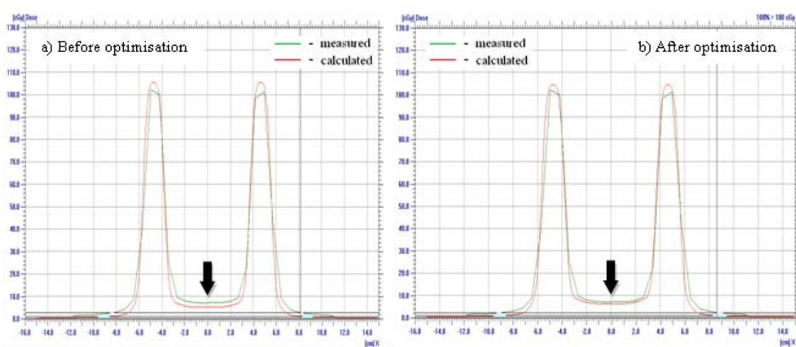
**Fig.3:** Profile 1 from the “Chair” test for 6 MV for depth 3 cm – a) before optimization, b) after optimisation.
