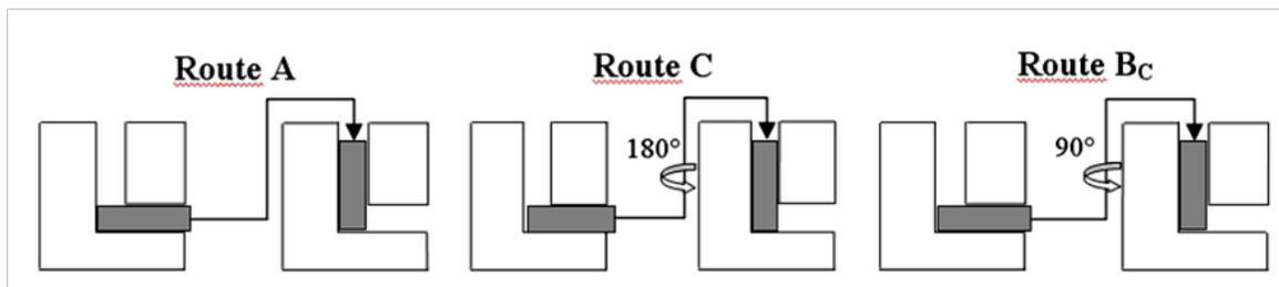
Fig. 5: Scheme of the processing routes in ECAP.
