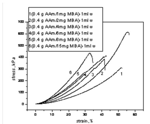
Fig. 1: Strain versus stress curves of AAm/MBA hydrogels
