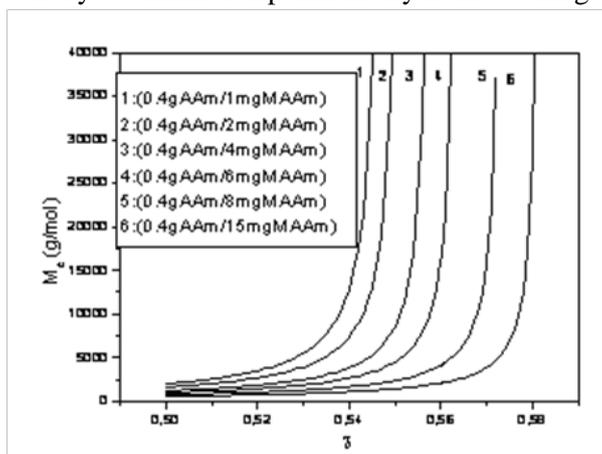
Fig. 3: The change of  $\overline{M}_c$  with  $\chi$  value of AAm/MBA hydrogels.
